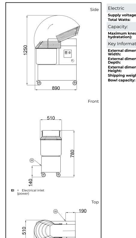
Electric Supply voltage: 380-415V/3 ph/50 Hz **Total Watts:** 2.2 kW Capacity: Maximum kneading (60% 33 kg/Cycle hydratation): Key Information: External dimensions, Width: 510 mm External dimensions, 840 mm Depth: External dimensions, Height: 780 mm 109 kg **Shipping weight:**
